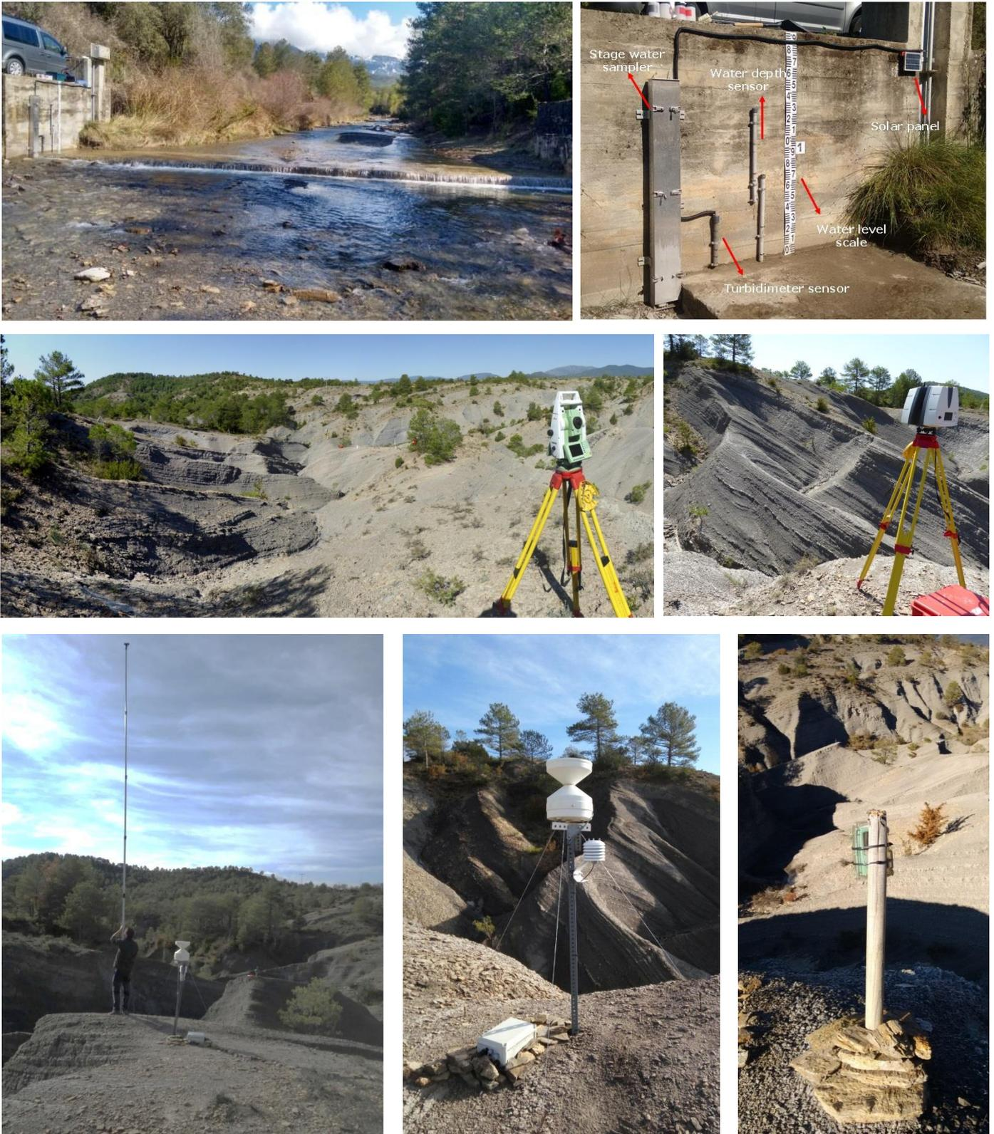
**Figure 2.** Some examples of data acquisition and instrumentation in the monitoring stations of the Soto Experimental Catchment (southern Pyrenees; the Upper River Cinca). Top: The outlet station. Middle: acquiring topographic data in Badland 1. Bottom: a new pole to acquire aerial imagery, the improved rainfall and air temperature station located in Badland 1, and an example of one of the time-lapse cameras installed, in this case, in Badland 1 (see Figure 1 for location).
