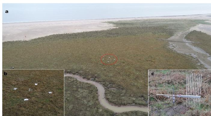
**Figure 1:** Location (a) and setup (b) of the RSET-MH installation on the "New Saltmarsh" in the Gibraltar Point National Nature Reserve, and the RSET measurement setup (c).
