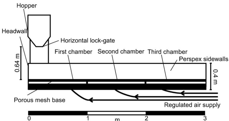
**Figure 1** Flume design, from Smith et al 2018
