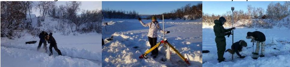
**Figure 1.** Drilling (left), ADCP setup of flow measurements (middle), GPS and ADV measurements (right).
