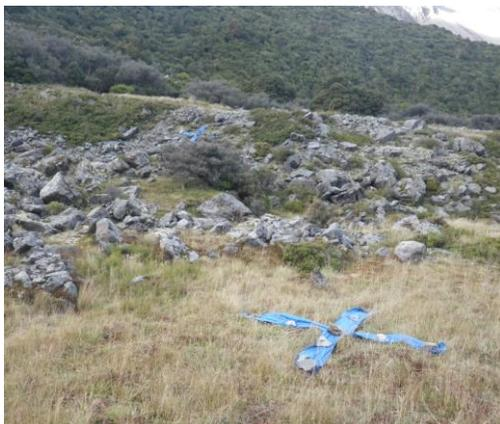
**Figure 1:** Ground control points set up with blue tarpaulin along the channel for SfM image acquisition.
