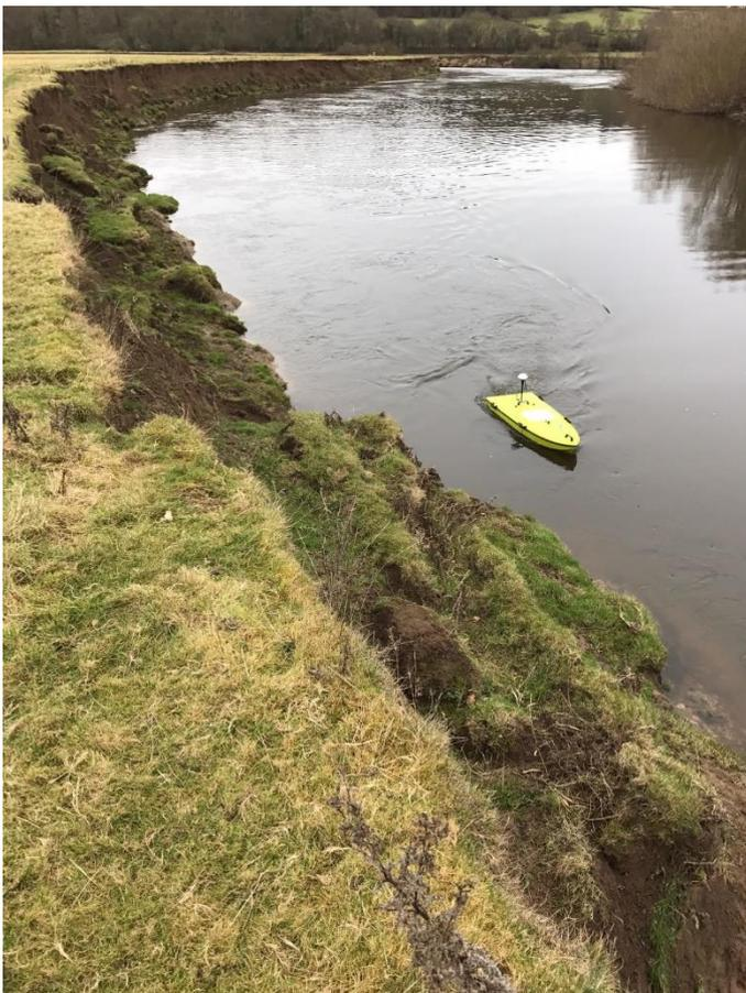
**Figure 1:** Collecting ADCP transects of near-bank flow velocities at low flow in March 2017.
