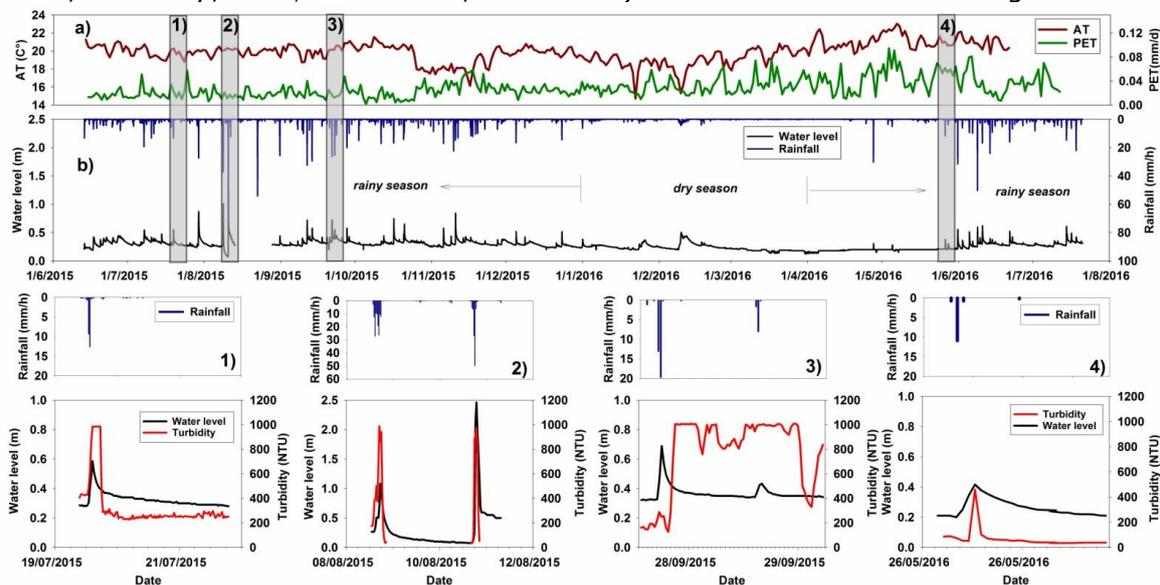
**Figure 2** a) hourly average air temperature (AT) and potential evapotranspiration (PET) estimates combined with b) the hourly rainfall-water level relationship are shown for four selected water level-turbidity events over the first year of monitoring.
