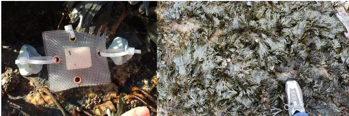
Figure 1 (left): limestone sample (5 x 4 x 1 cm) attached to rock platform.
