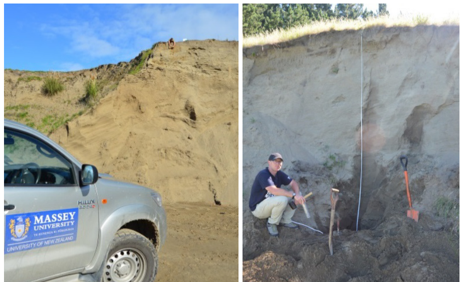
Figure 2: (left) Eastern-most dune ridge, with a recently excavated section, with OSL sample being recovered from the crest; (right) a section of the next youngest ridge, with OSL sample recovered from the base of the dune.
