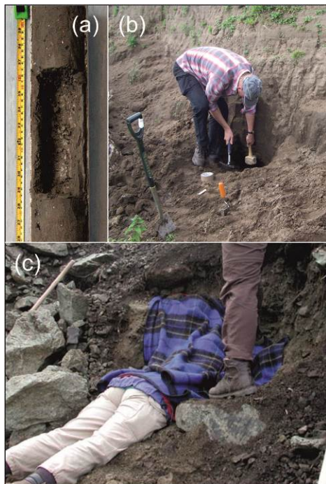
Figure 4: (a) An example of a luminescence sample taken from a core. (b) Sampling an exposed section by hammering a cylinder into the face. Photograph courtesy of Richard Chiverrell. (c) An opaque fabric or liner can be used to minimise exposure to daylight. Photograph courtesy of Barbara Mauz.
