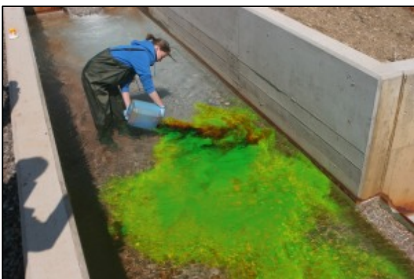
Figure 5. Photograph showing injection of a fluorescent tracer into a channel (courtesy: http://www.openchannelflow.com/blog/archives_article ).
