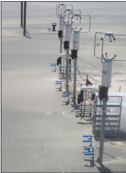
Figure 1: Field deployment of Wenglor photoelectronic fork laser sensors (blue), miniphones, vertical stack of hose trap, and 3-D ultrasonic wind anemometers.
