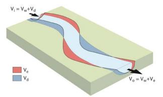
Figure 2: Application of morphometric method in fluvial geomorphology using equation 3. Vi and Vo are the volumetric sediment input and output. Vw is the volumetric washload material. Ve and Vd are the volumetric sediment erosion and deposition. Based on Church (2006).
