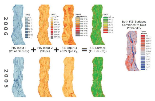
Figure 5. Example of mapping spatial variability of DEM of Difference (DoD) uncertainty using multiple parameters. For each DEM (2005 and 2006) the three inputs (point density, slope and GPS quality) are combined in a three rule fuzzy inference system to produce a defuzzified prediction of elevation uncertainty (where a probability > 0 is deposition and < 0 is erosion). Reproduced, with permission, from Wheaton et al. (2010: Figure 7).
