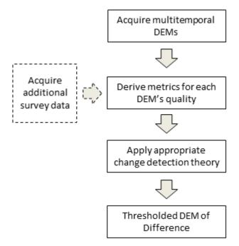
Figure 3: Workflow for DEM differencing with error assessment.
