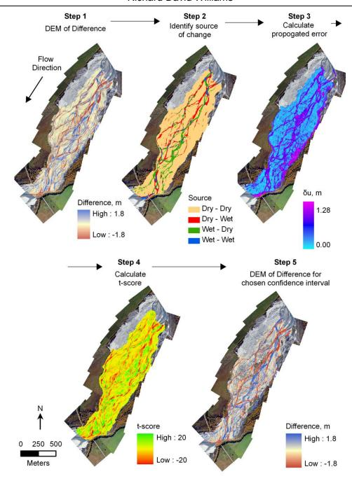
Figure 4: Workflow for producing a DEM of Difference by applying probabilistic thresholding using a user defined Confidence Interval. Reproduced, with permission, from Williams et al. (2011: Figure 8).
