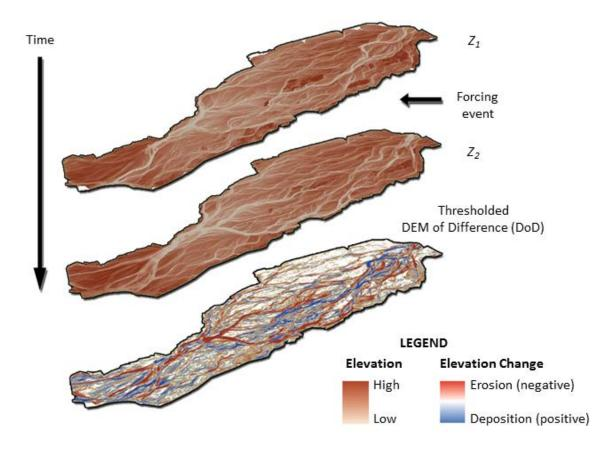
Figure 1: Thresholded DEM of Difference using data from the ReesScan project (Williams et al., 2011). For illustration clarity, DEMs have been detrended by subtracting the streamwise bed slope from each DEM. Approximate flow direction is from right to left.
