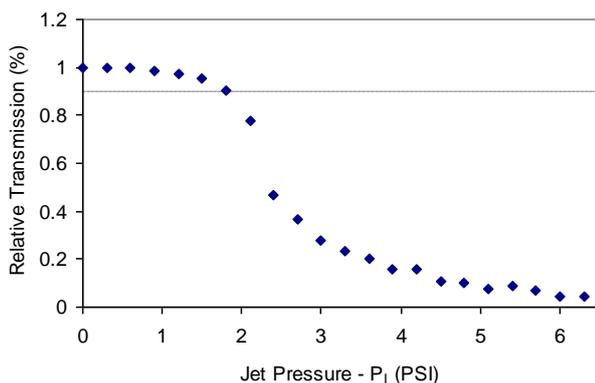
Figure 5: An example of a transmission curve from a cohesive strength meter run. A 10% reduction in transmission was used as the operation definition of erosion.
