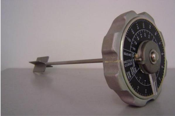
Figure 2: A shear vane tester equipped with a 33 mm diameter vane. The vane is inserted into the sediment, and the dial is rotated until the sediment fails, and the vane spins freely in the sediment.
