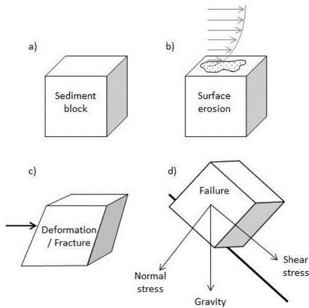
Figure 1: Shear stress imposed on a block of sediment resulting in (b) surface erosion, (c) sediment deformation / fracture, or (d) slope failure
