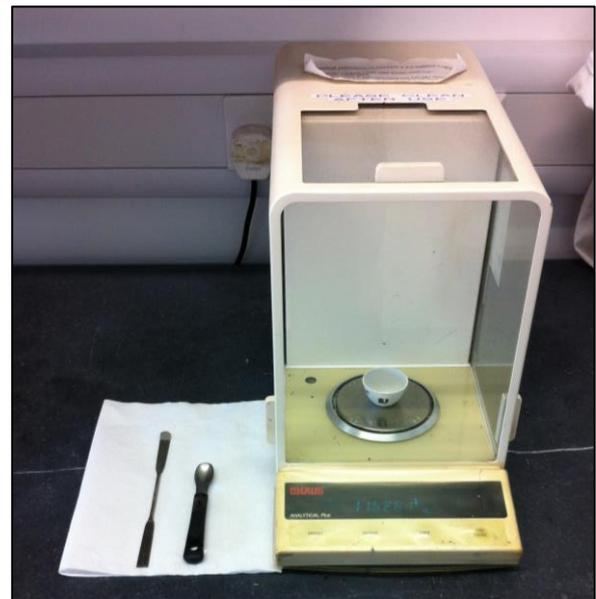
Figure 3. Obtaining crucible mass using a 4.d.p balance. Sampling spatula (left) and 1.25 cm<sup>3</sup> measuring spoon (right) included.
