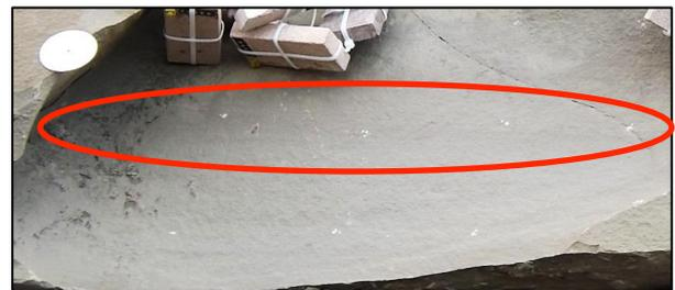
Figure 4: Impact damage from Schmidt Hammer (photo: Lisa Mol).
