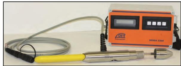
Figure 8. Ott electromagnetic current meter (Turnipseed and Sauer, 2010).
