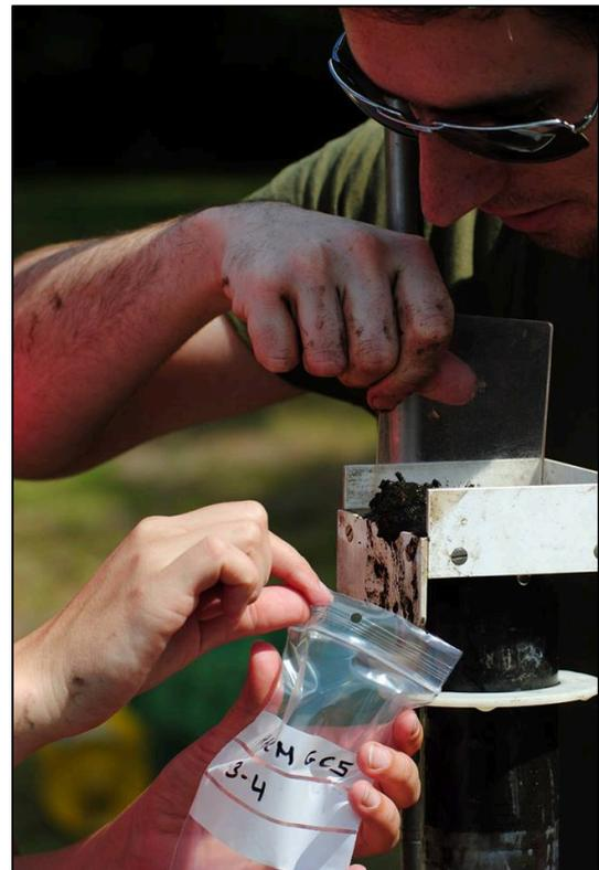
Figure 4: Subsampling of a surface core at Hämelsee, Germany, using an extruder device. Photography courtesy of W. van der Bilt.
