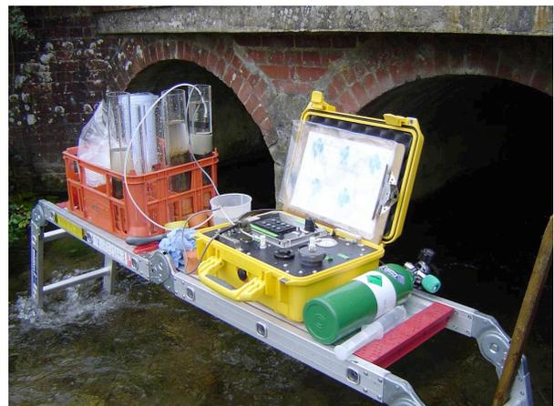
Figure 4: The cohesive strength meter (CSM) being used in the Bere Stream (Dorset, UK).
