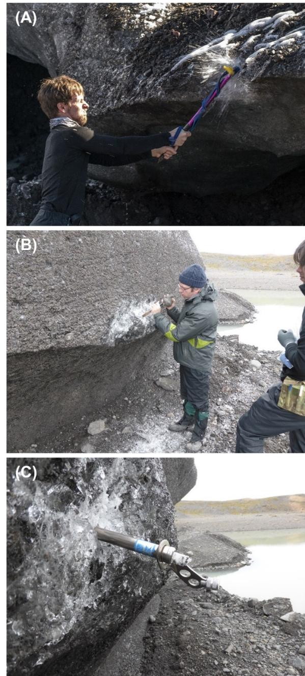
Figure 5: Ice sampling techniques using (a) an ice axe; (b) a chisel; and (c) an ice screw.
