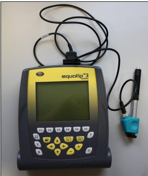
Figure 5: Equotip with impact device (right). Photo: Lisa Mol.
